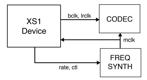
The xCORE device provides control to the frequency synthesizer and the frequency synthesizer provides the audio master clock to the CODEC and xCORE device. The sample bit and word clocks are then provided to the CODEC by the xCORE device.
