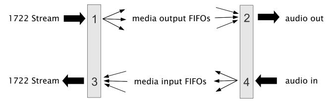
As described in the previous section, an IEEE 1722 audio stream may consist of many channels. These channels need to be routed to particular audio I/Os on the endpoint. To achieve maximum flexibility the XMOS design uses intermediate audio buffering to route audio.
